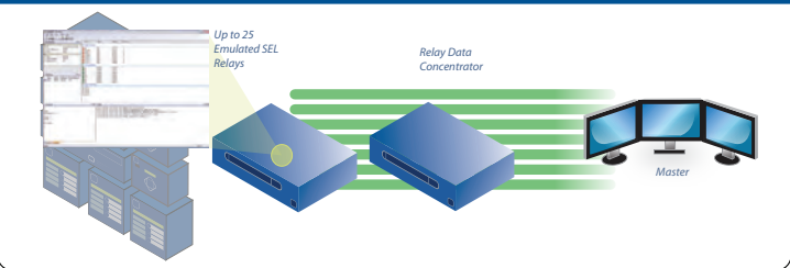
Step 3: Connect SUBNET SELRDE to Data Concentrator and enable emulation of up to 25 relays
